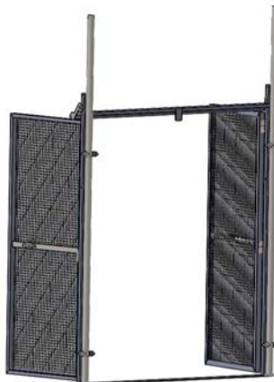
Standard Landing door Interlocked (no opening if the cage is not at the floor)
