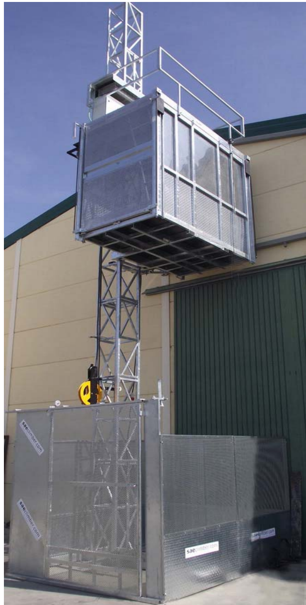
Standard Landing door Interlocked (no opening if the cage is not at the floor)
